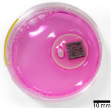
Bon30ID™ model (gray) attached to a bioreactor substrate, in a petri dish with cell culture medium (pink).
